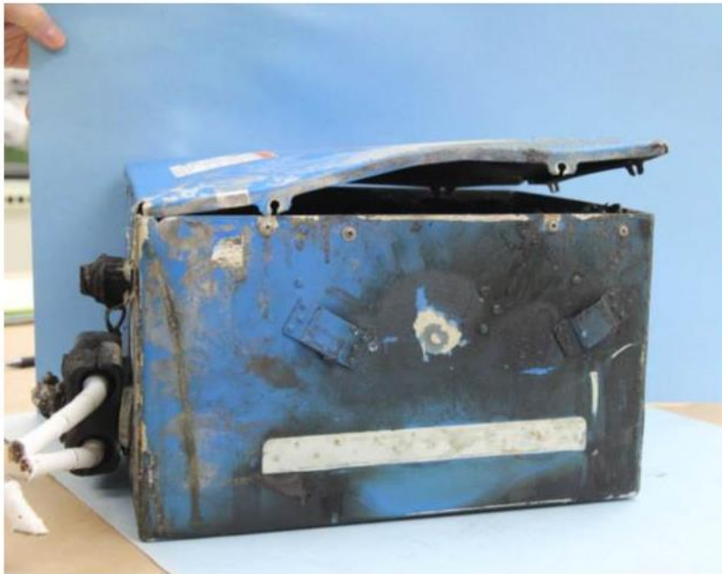
Figure 6. Right aft corner of the battery lid and side 4 of the battery case.
