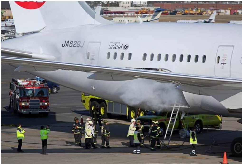
Figure 1. Photograph of smoke emanating from the incident airplane's aft E/E bay.
