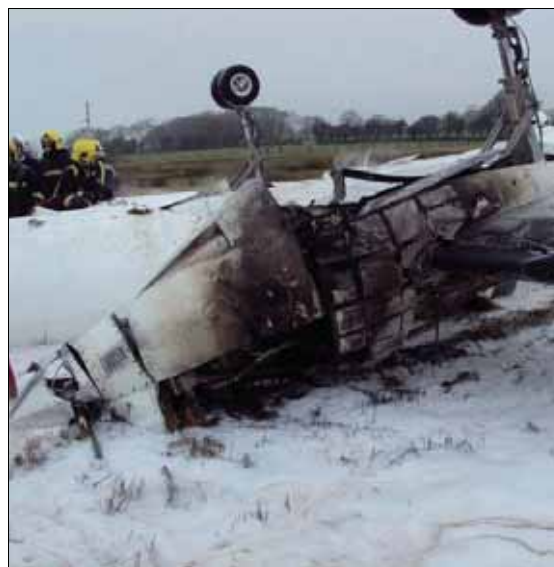
Photo No. 10: Right Engine Fire damage
