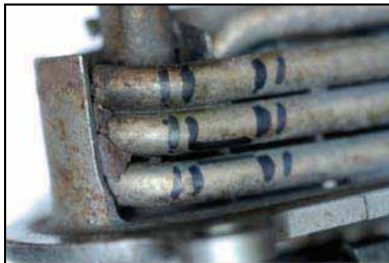
Photo No. 6: Possible sensing tube breach location
