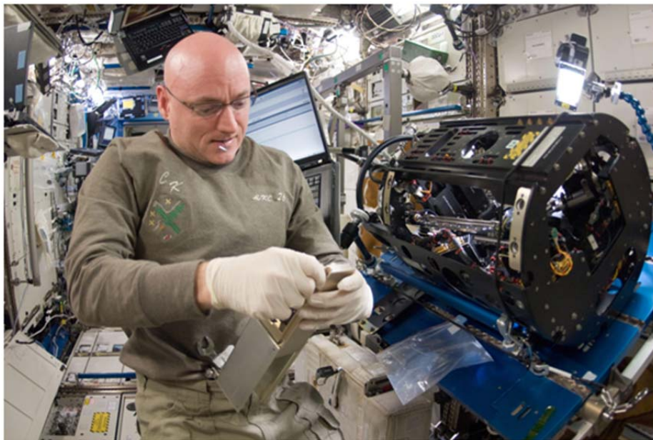
Figure 8. Astronaut working with the Combustion Integrated Rack Multi-user Drop Combustion Apparatus in the Destiny Lab of the ISS
